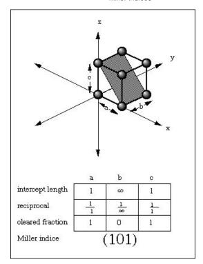
This becomes immediately apparent when we consider the <u>case of the (101)</u>. In this case the plane intercepts the a axis at one unit length and also the c axis at one unit length. The plane however, never intersects the b axis. In other words, it can be said that the intercept to the b axis is infinity. The intercepts are then designated as 1, infinity, 1. The reciprocals are then 1/1, 1/1 infinity, 1/1. Knowing 1/1 infinity = 0 then the indices become (101).
