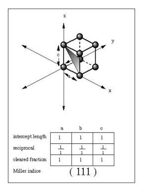
If you want to describe the orientation of a crystal face or a plane of atoms within a crystal lattice, then there are series of steps that will lead you to its notation using Miller indices.
