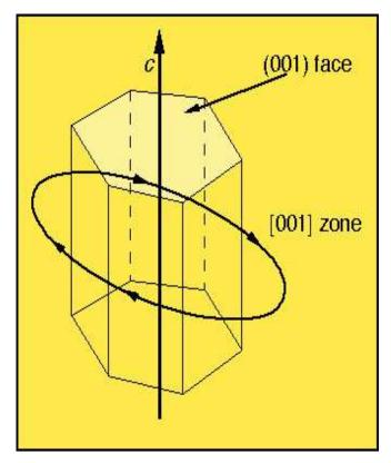
Only in the isometric systems are the same integers used to relater the perpendicular to a family of planes (hkl) to the directions [uvw].
